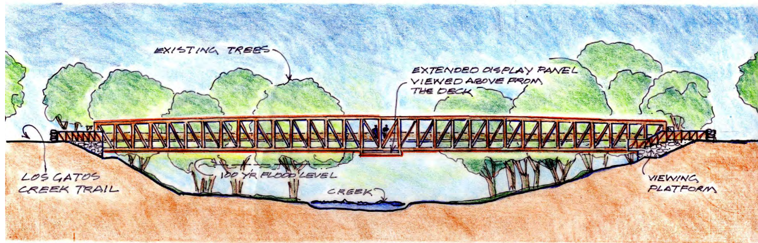
ELEVATION OF SCHEME FIVE FOR LOS GATOS CREEK . JULY-AUG. 6/13 BRIDGE REPLACEMENT . SAN JOSE . CALIF. AM/12
