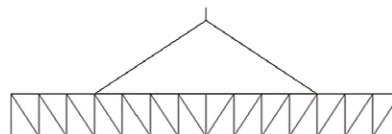
Fully Assembled Truss Only (top chord lift)
